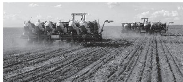
Figure 20-15. Four- (top) and six-furrow (middle and bottom) cassava planters.
