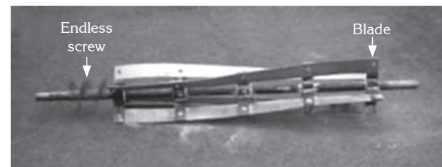
Figure 23-5. A mill shaft.
