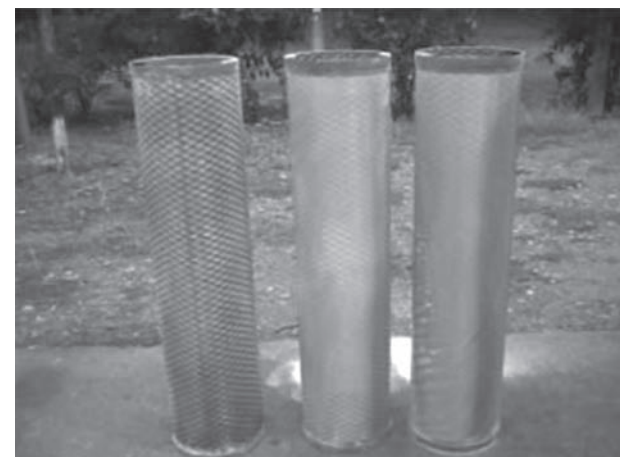
Figure 23-6. Sieves for milling and classification, with mesh openings of, from left to right, 3 mm, 177 μm, and 100 μm
