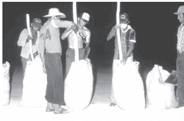
Figure 21-10. Tamping down dried chips in sacks. Sacks weighing over 50 kg can then be obtained.
