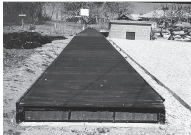
Figure 22-2. The solar collector used to heat air for a cassava chip dryer.
