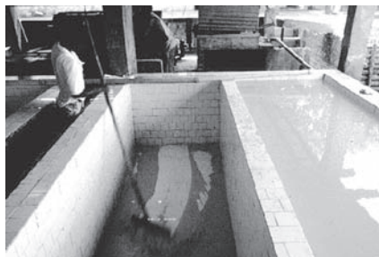
Photo 26A-4. Sedimented starch in tanks (the worker is separating the black starch).
