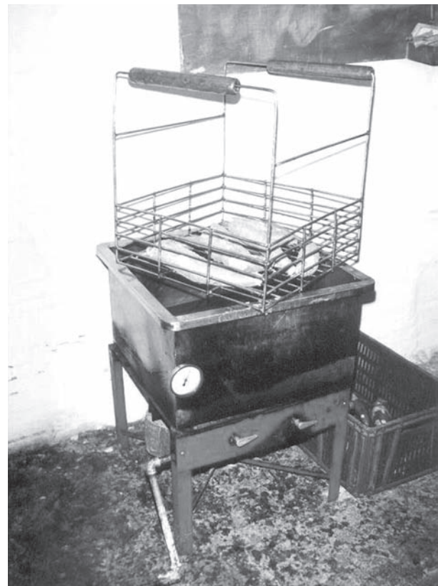
Figure 25-20. Steel rod basket that holds from 2 to 3 kg of fresh cassava roots, used during paraffin treatment.
